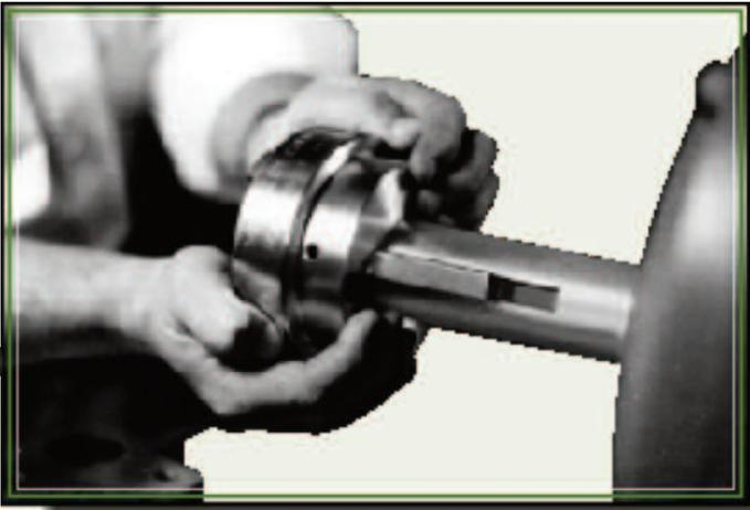
**Shaft spacing** should be within range given by dimensions 'W' and 'X' as shown in charts on page 4.
